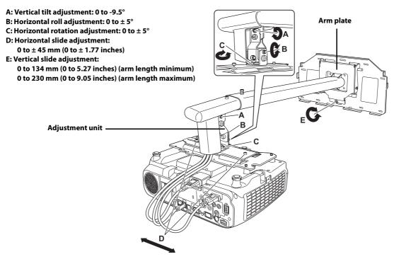
5) Firmly tighten the screws on the arm unit and adjustment unit using the hexagonal wrenches (M4 and M8).
